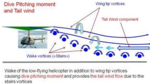
Fig. (20). The flow pattern in the wake from a low-flying helicopter.
