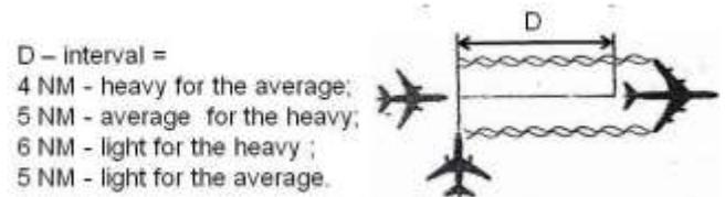
Fig. (25). Acceptable intervals between aircraft moving in the air.
